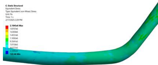
Fig. 5(c). Stress distribution inside the 135° elbow: v=4 m/s.
